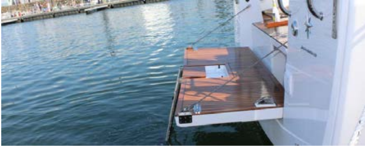
Sloped telescopic ladder for a better access on board, handrail and access step to the cockpit
