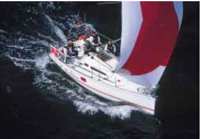
**THE SUN FAST 26** creates on its own the desire to go sailing, thanks to the fast hull design from Philippe Briand. It is proportionally as wide as today's bigger ocean racing boats. It has the following advantages that allow it to quickly reach and surpass hull speed : twin rudders, gennaker with bowsprit, bulb keel, full-roach mainsail. The SUN FAST 26 already surfed to the top of the sailboat market.
