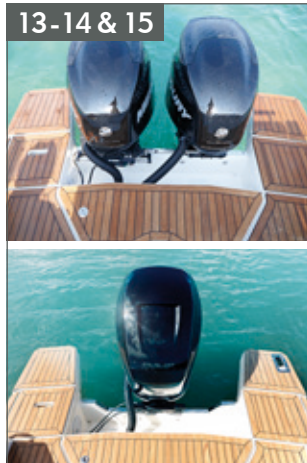
Double swim platform Motor well bridge: easy access to both sides of transom Single or twin engine configuration capability of max 400 hp
