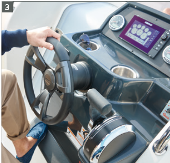
Stylish and ergonomic bicolor helm with integrated cup holders, storage tray and mounting space for optional 7" GPS/Chart Plotter
