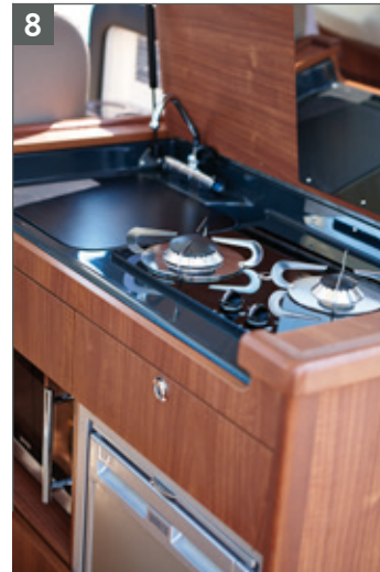
Galley with pressure water, LPG stove and optional refrigerator and microwave
