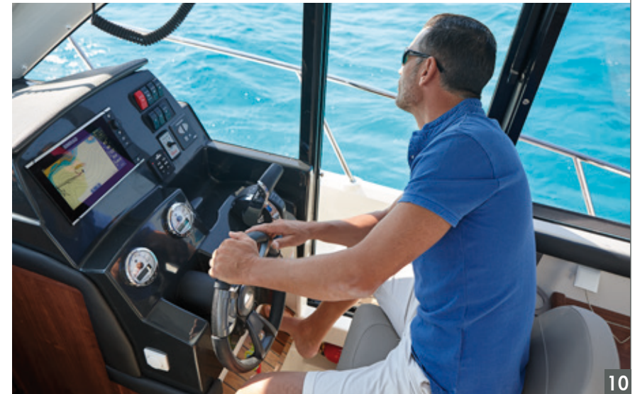
Integrated helm with SmartCraft instrumentation, mounting area for optional GPS/Depthfinder/stereo
