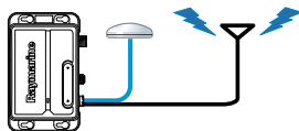
AIS650 class B AIS transceiver Receive and transmit AIS navigation status information on e series. Use the VHF antenna. Raymarine part number : E32158
