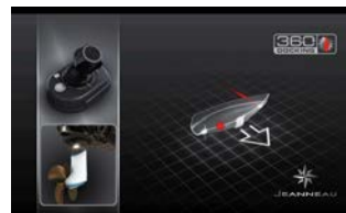
> Sideways movement: saildrive turns 90° and activates bowthruster
