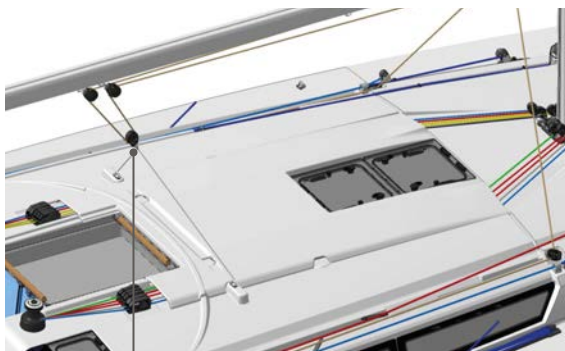
Here is the track system used by Sun Odyssey 449. Putting the boom in the axis requires adjustment of the track with each tack.
