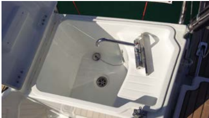
Cockpit sink with hot & cold water
