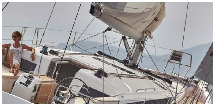
Y-bridle system used by the Sun Odyssey 490. By bringing the pulleys closer to the boom, the bridle allows for good boom angulation, similar to that of a Mainsail track without any adjustments to be made during the tacks.
