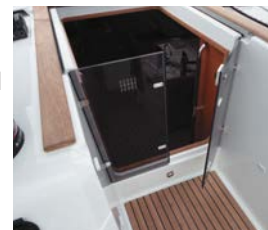
Companionway hatch with hinged double doors
