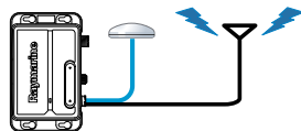
AIS650 class B AIS transceiver Receive and transmit AIS navigation status information on e series. Use the VHF antenna. Raymarine part number : E32158
