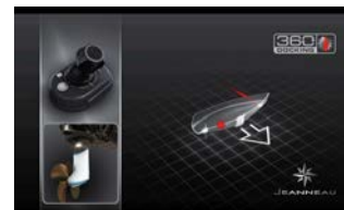
> Sideways movement: saildrive turns 90° and activates bowthruster
