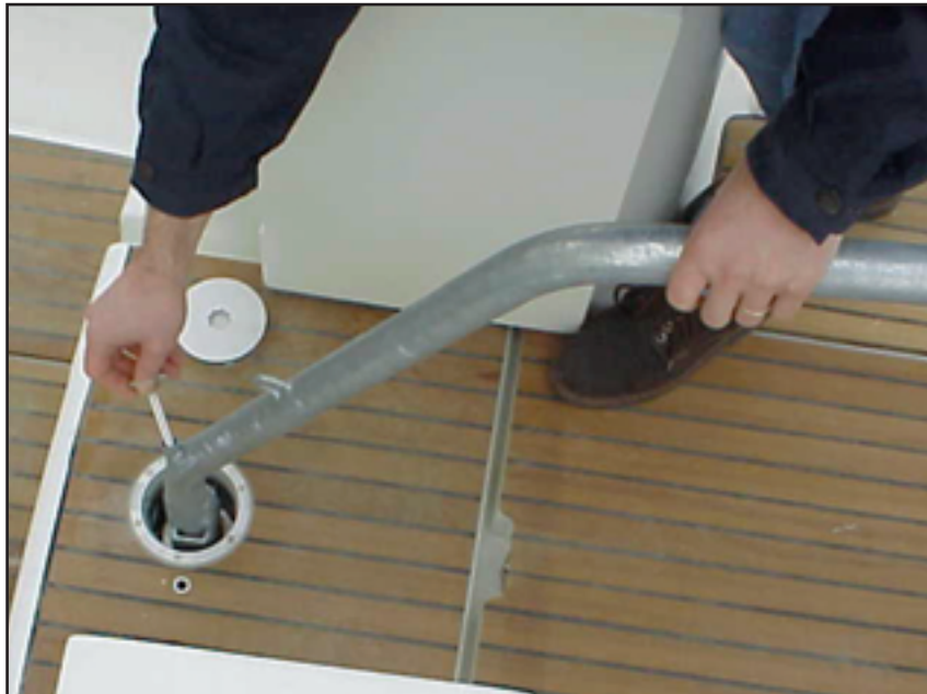
Overtightening with bolt
