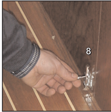
8 - Unlock the bolt at the foot of the bulkhead.
