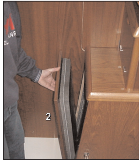
2 - Remove the starboard engine trap door.
