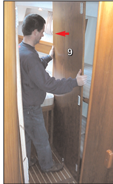
9 - Dislodge the lateral bulkheads. These bulkheads are broached together. Put them aside.
