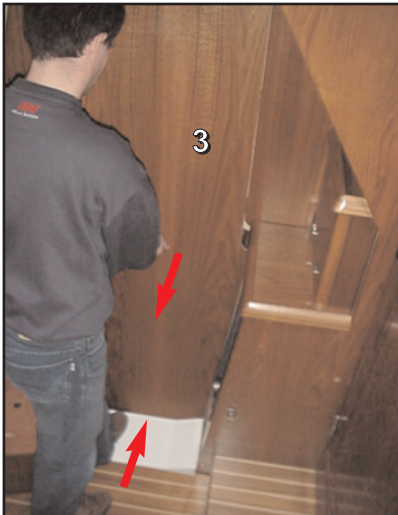
3 - Dislodge the central bulkhead (fixed with «velcro») pulling the handle.
