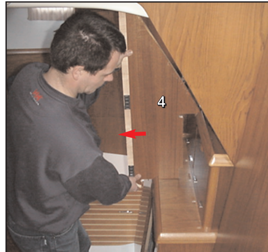
4 - Dislodge the bulkhead section above engine.
