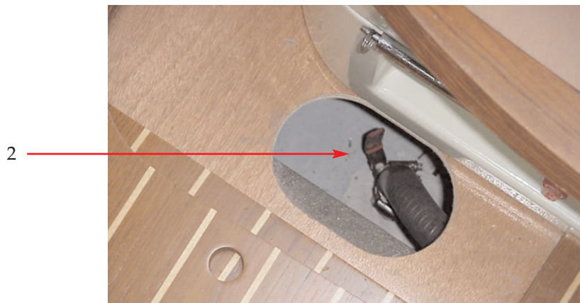
2 - Engine sea-water valve, seacock with valve
