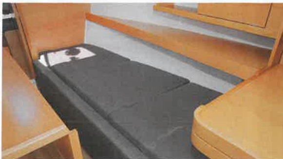
Lift off the settee seatbacks, hang them on the front of the seat and you're left with a comfortably wide and long berth on each side
