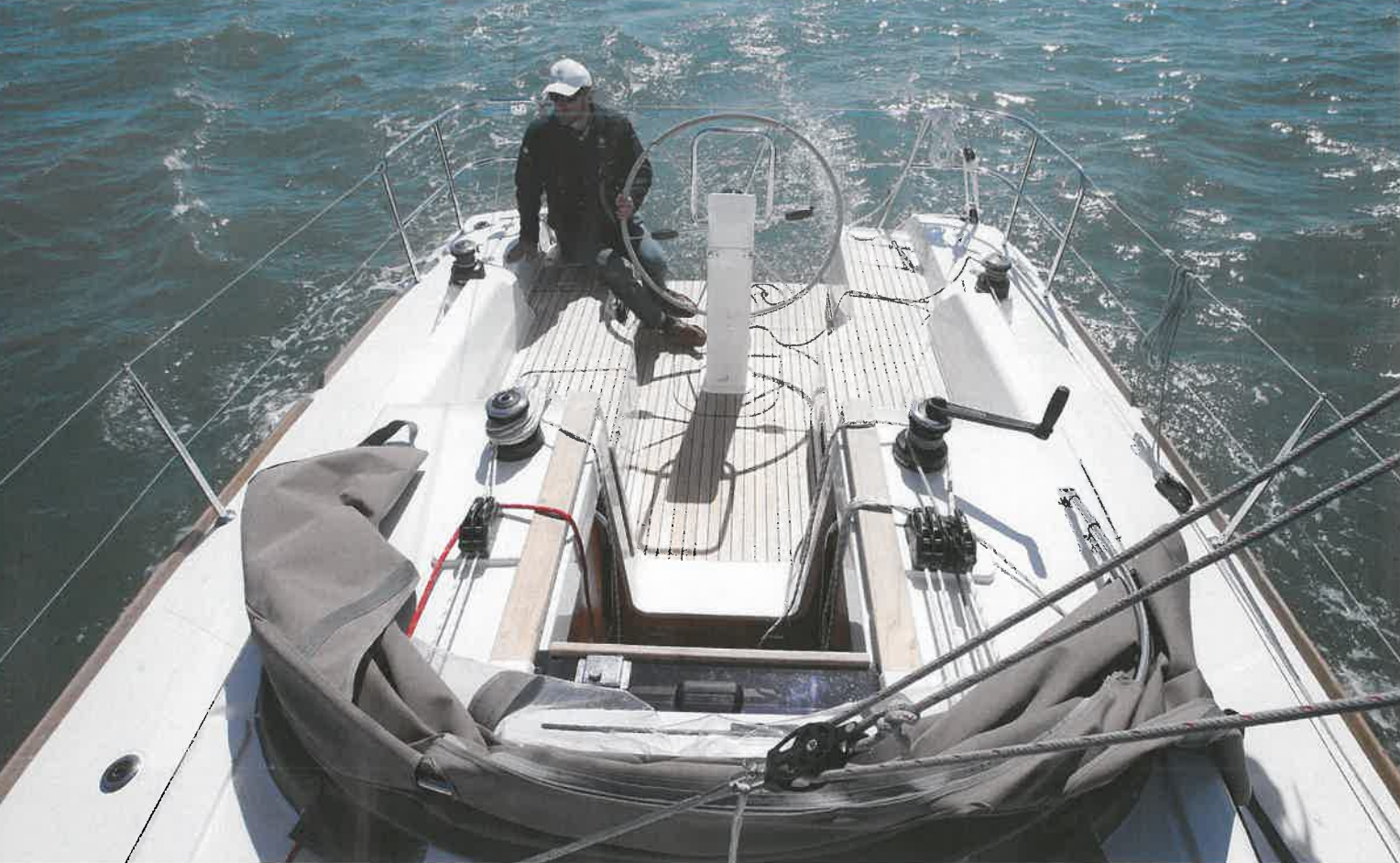
ABOVE: A clean and sensible cockpit. For shorthanded sailing, leading the mainsheet back to the helm would be a good idea BELOW: A high coach roof makes space below decks
