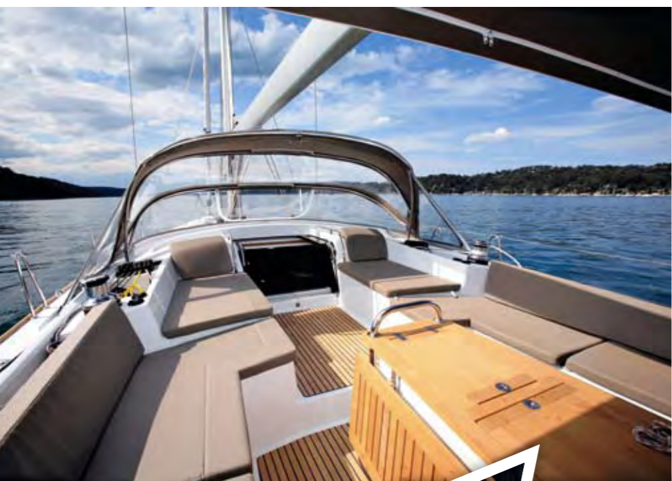
No need for crew and guests to get tangled up underway, such is the size of the massive cockpit, which includes two separate seating areas (left). The drop-side table has a hatched sink and icebox (refrigerated on the test boat).
