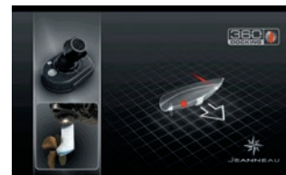
> Sideways movement: saildrive turns 90° and activates bowthruster
