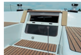
Companionway door slides into cockpit floor for easy storage
