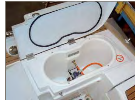
LOCKER / STORAGE SPACE FOR GAS BOTTLES
