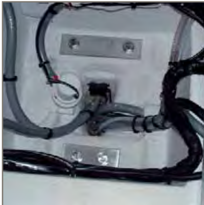
SALOON FLOORBOARD - ACCESS TO THE KEEL BOLTS
