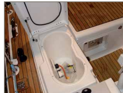
LOCKER / STORAGE SPACE FOR GAS BOTTLES
