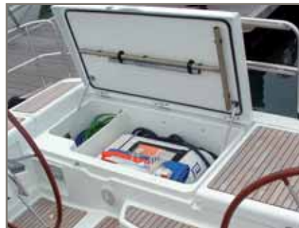
STORAGE SPACE FOR THE LIFE RAFT + EMERGENCY TILLER
