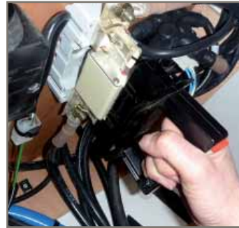
TAKING THE FUSE OUT OF THE THRUSTER - 1
