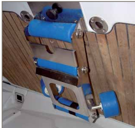
TENDER LOWERING RAMP
