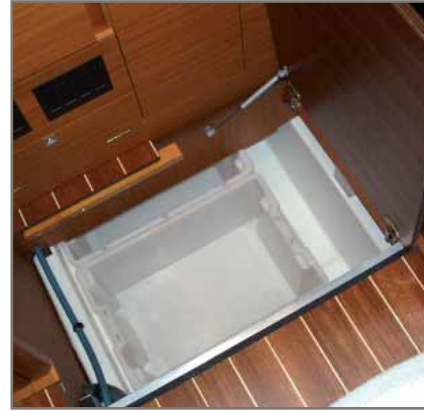
GALLEY FLOORBOARD - ACCESS TO THE STORAGE BOXES
