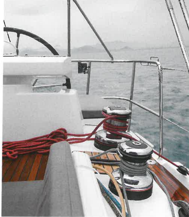
Above: the winch set up outboard won't suit all – it's designed for powered reversible winches or Jeanneau's AST system.
