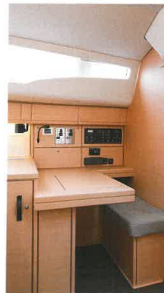
Left: all layouts, from two to five cabins, keep the dedicated navstation
