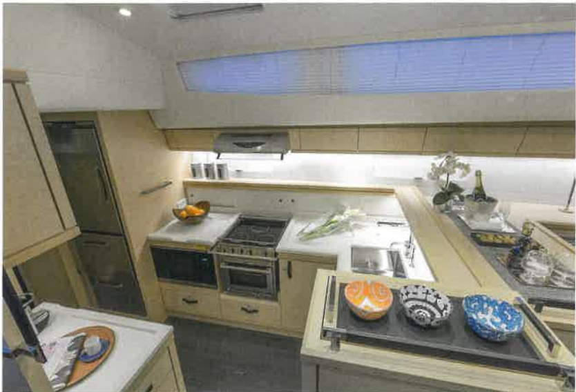
Galley: the passageway galley is secure to work in at sea, provides reasonable fiddled worksurfaces, plus plenty of dried goods stowage and options for cold stowage. It has been thoughtfully arranged to suit the idea of service, including stainless steel fridges and the siting of a cutlery drawer and drinks fridge close to the companionway. Raised locker and crockery space is limited, however
